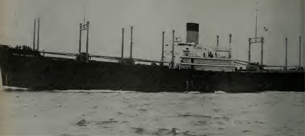
The Sea Skimmer. This is a typical C-3 and is one of the first of the type to be turned over to Matson for conversion. She has been renamed Hawaiian Merchant. Except for painting, changes in cargo handling equipment will be the most obvious difference.
